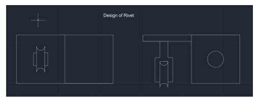
Figure 3. Design of Rivet for Net Installation
